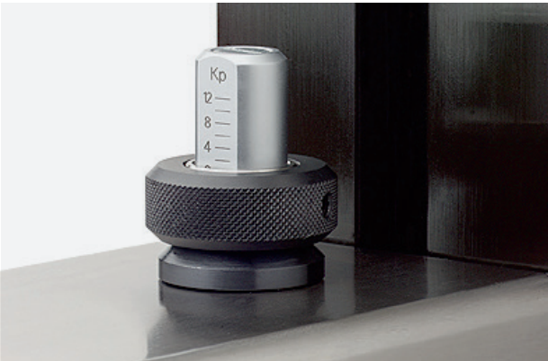
→ MDU 2: Setting of downward force for child-resistant bottle caps
